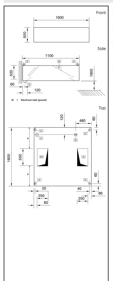
**Electric** Supply voltage: 220 V/1N ph/50 Hz **Total Watts:** 0.16 kW Capacity: Supply capacity: 1470 m<sup>3</sup>/h **Key Information:** External dimensions, Width: 1600 mm 1100 mm External dimensions, Depth: External dimensions, Height: 500 mm Net weight: 111 kg Air Emission:
